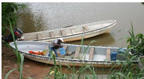
Figure 6. A fibreglass vessel with an 40hp outboard motor was used for most small-boat survey efforts. Advantages include it being fast, stable and manoeuvrable.
