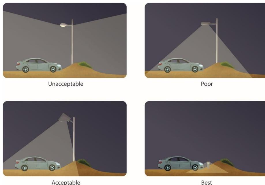
**Figure 14 Lighting options for a parking area. Figure adapted from Witherington and Martin (2003).**
