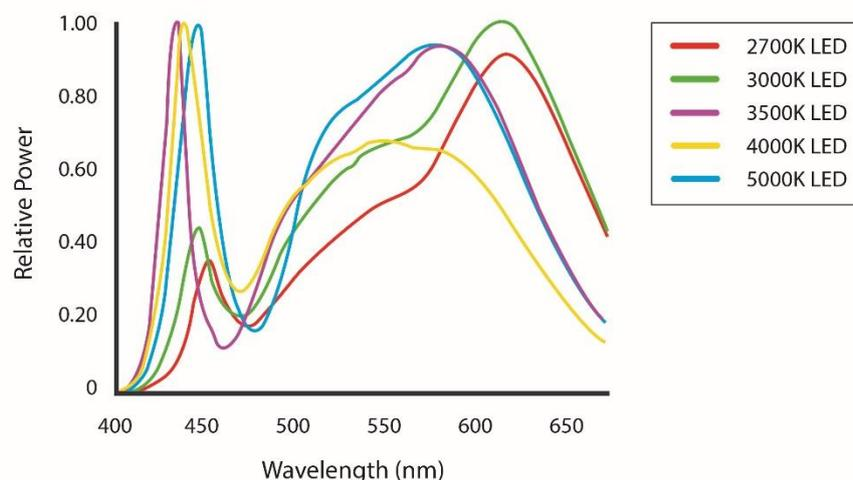
**Figure 23 Spectral curves showing the blue content of white 2,700-5,000 K LED lights. Note the difference in relative power output in the blue (400 - 500 nm) wavelength range. Figure courtesy of Ian Ashdown.**
