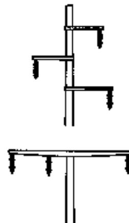
lines/wires should be spaced at least 140 cm apart. Hardware that is used to prevent arcing (“St. Elmo's fire” on both sides of the insulators) should not be used.
