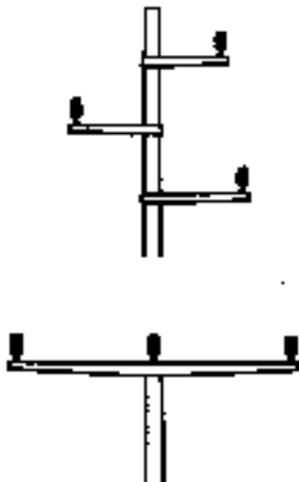
Power poles with upright insulators are widely used and rank as the most dangerous of all types. The gap between the power lines and the crossarm is small, in older structures the lines run along the side of the top of the power pole.
